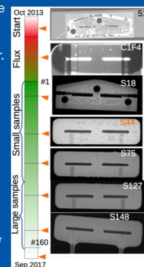
Figure 5: Evolution of the fluidic connector soldering technique.
