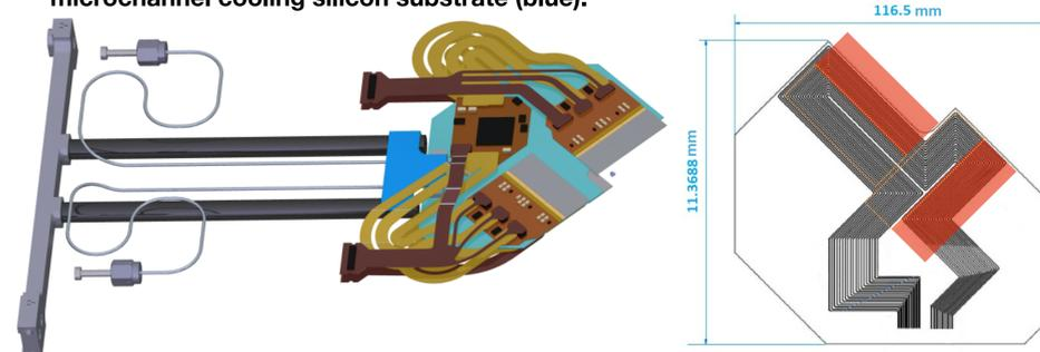
Figure 2: The VELO Upgrade Module. The design including all of the electronic element (left). On the right the microchannel design marked with the sensor positions (red).
