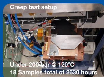
Figure 4: Plastic deformation due to low mechanical stress (creep) and the setup used to test both creep effect and fatigue.
