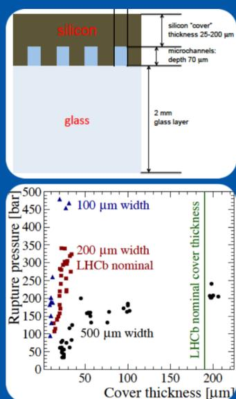
Figure 3: Scheme of samples for rupture test (top) and results of observed ruptures (bottom). No ruptures were observed in nominal LHCb samples.
