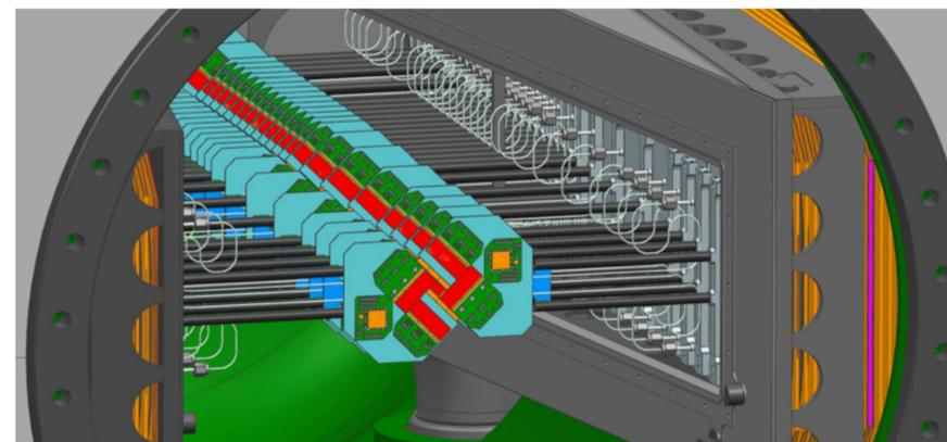
Figure 1: The VELO Upgrade. Each module has four sensors (in red) on a microchannel cooling silicon substrate (blue).
