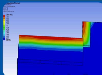
Figure 6: Thermal simulation of the VELO module.
