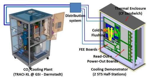
Bi-Phase CO<sub>2</sub> cooling at -25°C for FEE (40kW in ~2m<sup>3</sup>)
