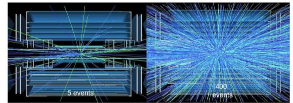
↑ Difference between low luminosity and high luminosity experiments at LHC. For high luminosity experiments, reducing pile-up becomes an important issue
