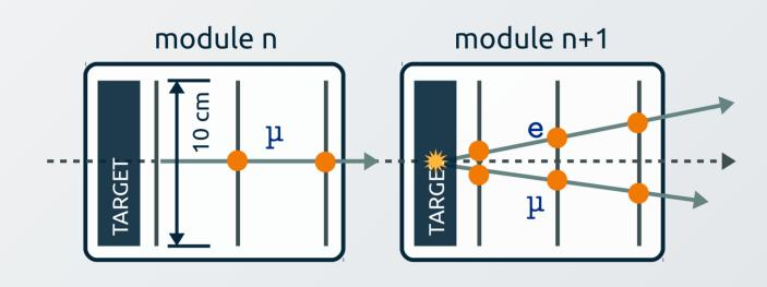
A modular target is foreseen in the final setup, consisting of 60 low-Z layers each sandwiched in layers of Si-microstrip detectors
