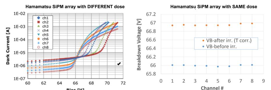
A Hamamatsu 8 channel array was radiated with different doses for each pixel (1E12 to 2E14). We found a linear behavior vs dose of up to 4 volt shift at highest dose. The 15 micron HE SiPM array radiation at 5E13 n/cm2 for all 8 channels shows very uniform behavior of the breakdown voltage shift.
