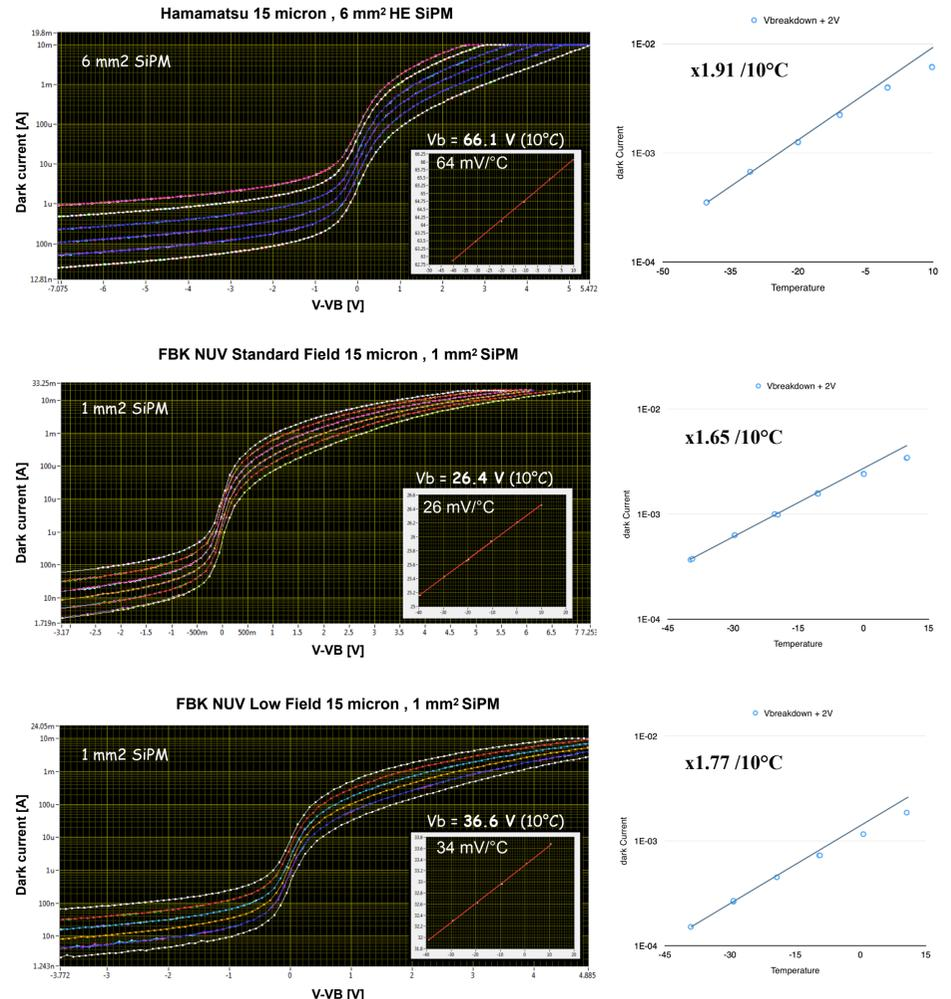
We observe a much weaker dependence on the dark current vs temperature of SiPMs with silicon based simple PIN diodes (typically 2.42/10°C). However we find different dependence of this behavior for SiPMs with different internal field (breakdown voltage). High Electric Field effects (such as tunneling and field enhanced generation) play a significant role in the SiPM dark noise.
