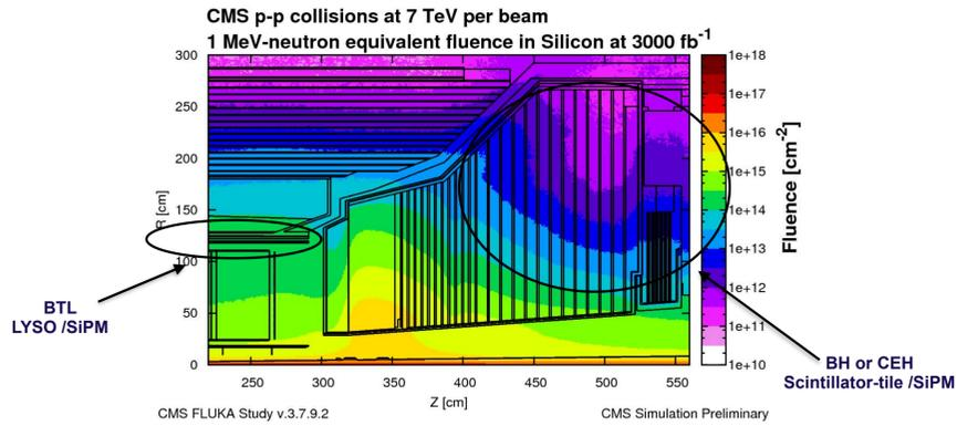
Two new projects in CMS called BTL (Barrel Timing layer) and BH (The Behind Hadronic Calorimeter) have proposed to use SiPMs as photodetector. The very high radiation damage environment of the proposed location in CMS is a challenge for operation of the SiPMs. However the proposed temperature of operation is -30°C.
