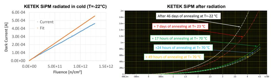
A KETEK 3x3 mm2 SiPM with peltier cooler was radiated at the CHARM facility at CERN at -22°C. The current was monitored during radiation. From the fit of the lower dose we can see that the current vs dose is nonlinear showing visible annealing even at -22°C
