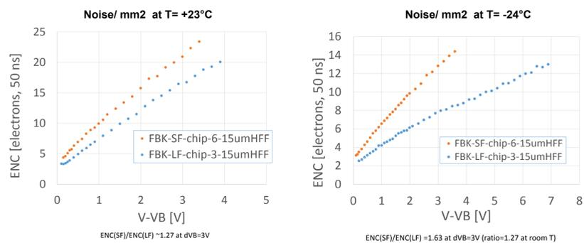
Comparison of noise between Standard field and Low field FBK SiPM after radiation at room temperature and low temperature. Much larger reduction in noise vs temperature was found for the low field SiPMs
