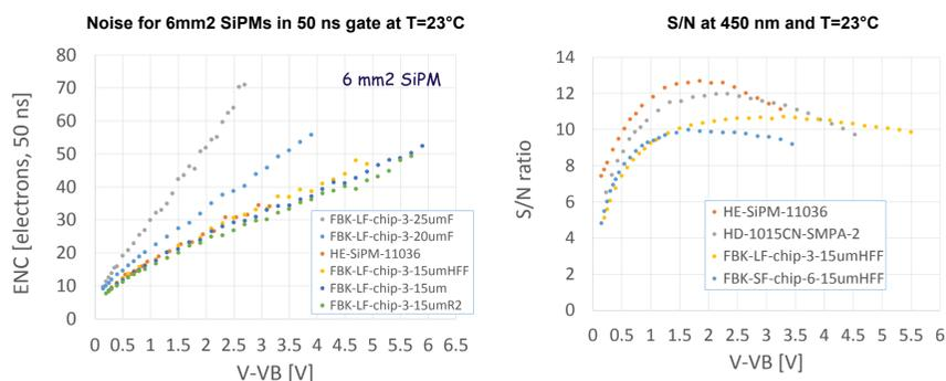
Noise and Signal over noise (S/N) at 450 nm after radiation in a 50 ns gate at room temperature. We found that the best operating point after radiation is around 2V over-voltage.
