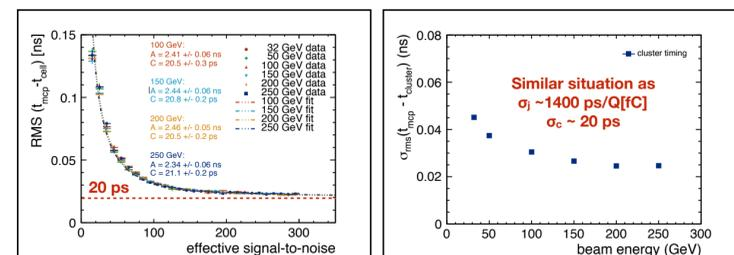
**Uncertainty vs S/N and beam energy after  $5.7 X_0 W$ :** Results are limited by electronic noise and MCP resolution.
