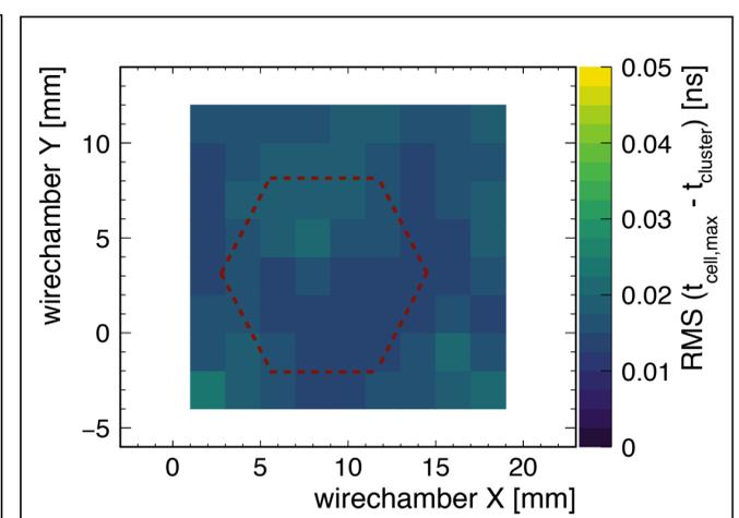
**Uncertainty vs. impact at 200 GeV,  $10 X_0 W+Pb$ :** Results are uniform across the illuminated sensor area. The red hexagon indicates the approximate position of the central pad.
