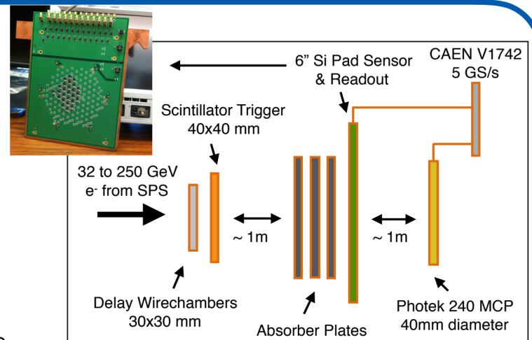
**Experimental Setup:** A silicon pad sensor with custom read-out optimised for timing tasks samples EM showers. Time differences between pads and relative to the MCP are analysed.
