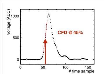
**Example silicon waveform:** Timestamp extracted at 45% of peak height.
