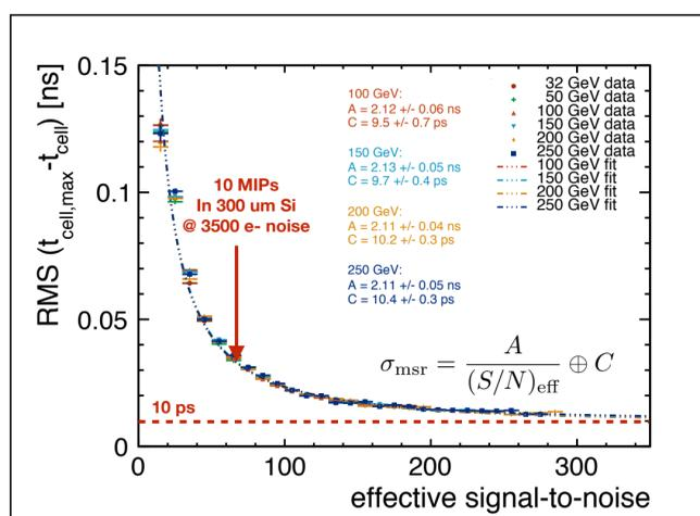
**Uncertainty vs. S/N after  $5.7 X_0 W$ :** Uncertainty is well modelled by a two parameter function, accounting for jitter (A) and constant (C) contributions.
