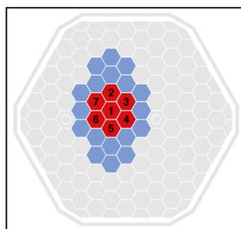
**Silicon pad sensor:** Only red cells are used for the presented data.
