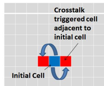
Fig. 3. Near-neighbour (Gallego) model, where microcells are triggered adjacent to the initial cell
