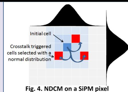
Fig. 4. NDCM on a SiPM pixel
