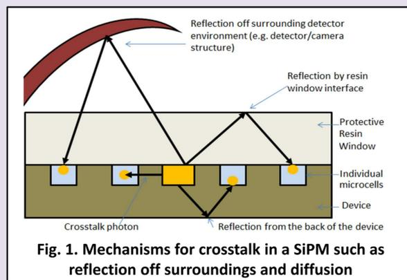
Fig. 1. Mechanisms for crosstalk in a SiPM such as reflection off surroundings and diffusion
