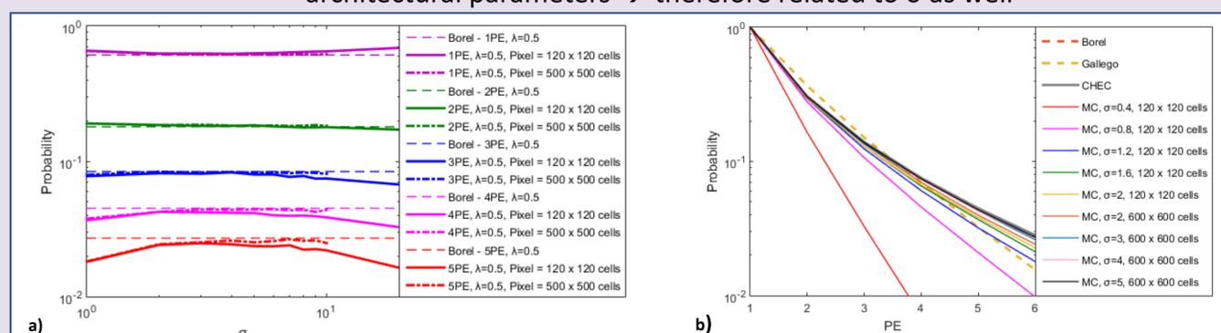
Fig. 5. a) PE probability as a function of  $\sigma$ , lower for higher PE as number of available cells is constrained. b) the CHEC-S data is approximated best for NDCM  $\sigma=5$
