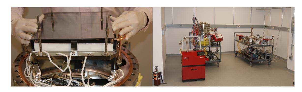
(*Left:*) Air-transfer of the window with pre-deposited layer of Sb. (*Right:*) University of Chicago PSEC Lab with two vacuum processing chambers. Due to their compact size, potentially many chambers could be operated at the same time at a future LAPPD production facility, using a shared vacuum distribution system. Each vacuum processing chamber could accommodate several LAPPDs. This batch production strategy would be similar to PMT batch production.
