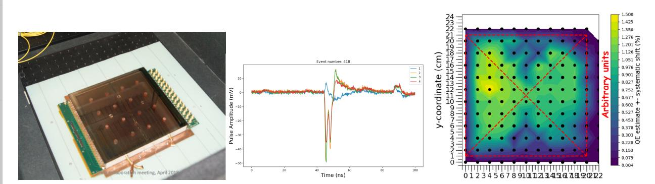
(*Left:*) Complete Gen-II LAPPD tile-21. (*Middle:*) Pulses from tile-21. (*Right:*) Final photo-sensitivity map of the tile-21 in arbitrary inits. Tile-21 was an early test of cesium transport. Improved photo-cathode uniformity is expected in future devices.
