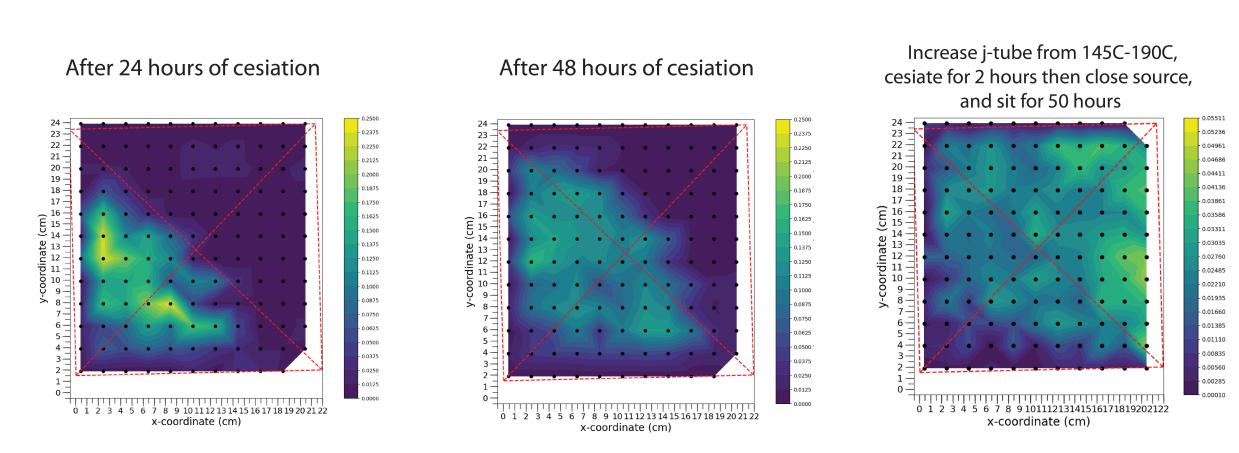
In-situ photo-cathode synthesis showing photo-sensitivity expressed in arbitrary units. Direct measurement of photo-current and absolute QE were precluded since the photo-cathode, MCPs, and the anode were interconnected with an internal high-voltage divider as part of a simplified strategy to power the tile (see Refs. 2-3). Future devices will allow direct measurement of photo-current and calibrated QE.
