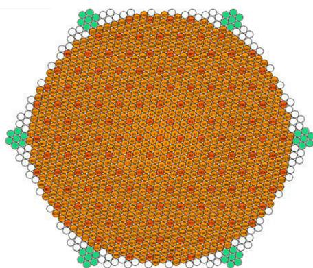
Left: Photo of a MAGIC camera; Right: PMT pixel positions in orange, open locations in green
