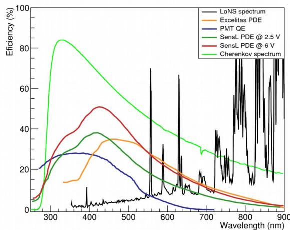
SiPM PDE of SensL and Exceiltas compared to the Cherenkov spectrum and the light of the night sky
