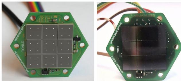
Left: Hamamatsu pixel Right: SensL pixel
