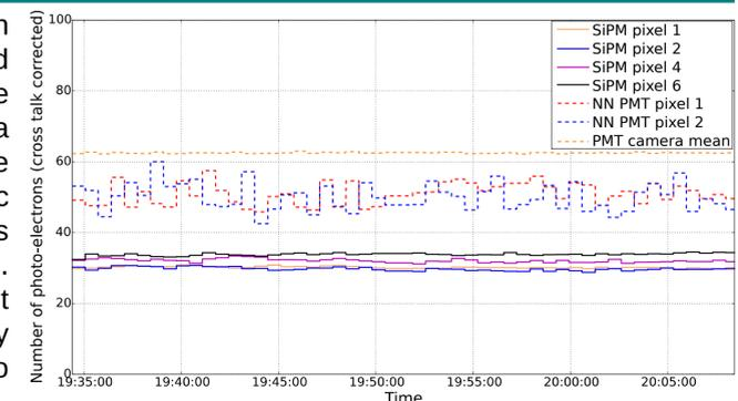
Detected number of photo-electrons of a Gen. 1 SiPM pixel compared to the performance of the next-neighbour (NN) PMTs and the PMT camera mean.
