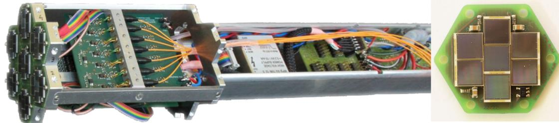
First generation SiPM module with opened cluster body. It holds 7 pixels each with 7 Excelitas SiPMs
