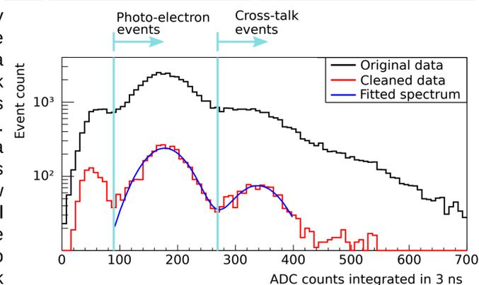
Unfiltered and filtered charge spectrum of a Gen. 1 pixel
