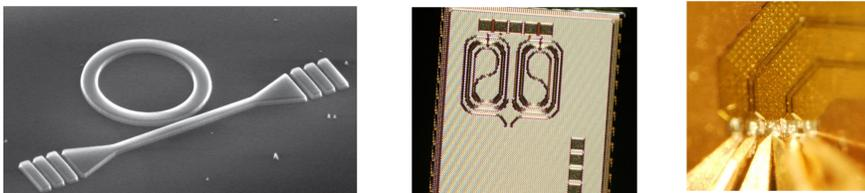
Optical modulation is obtained in silicon photonics circuits via electro-optical effect (plasma dispersion). In a MZI the electro-optical effect is used to modulate the interference condition of the two branches of the interferometer, while in a RR it is used to control the resonance condition of an optical ring coupled to an optical waveguide.
