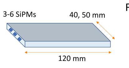
From the previous study about a timing counter Plastic scintillator : BC422, Saint-Gobain  $40,50 \times 120 \times 5 \text{ [mm}^3\text{]}$
