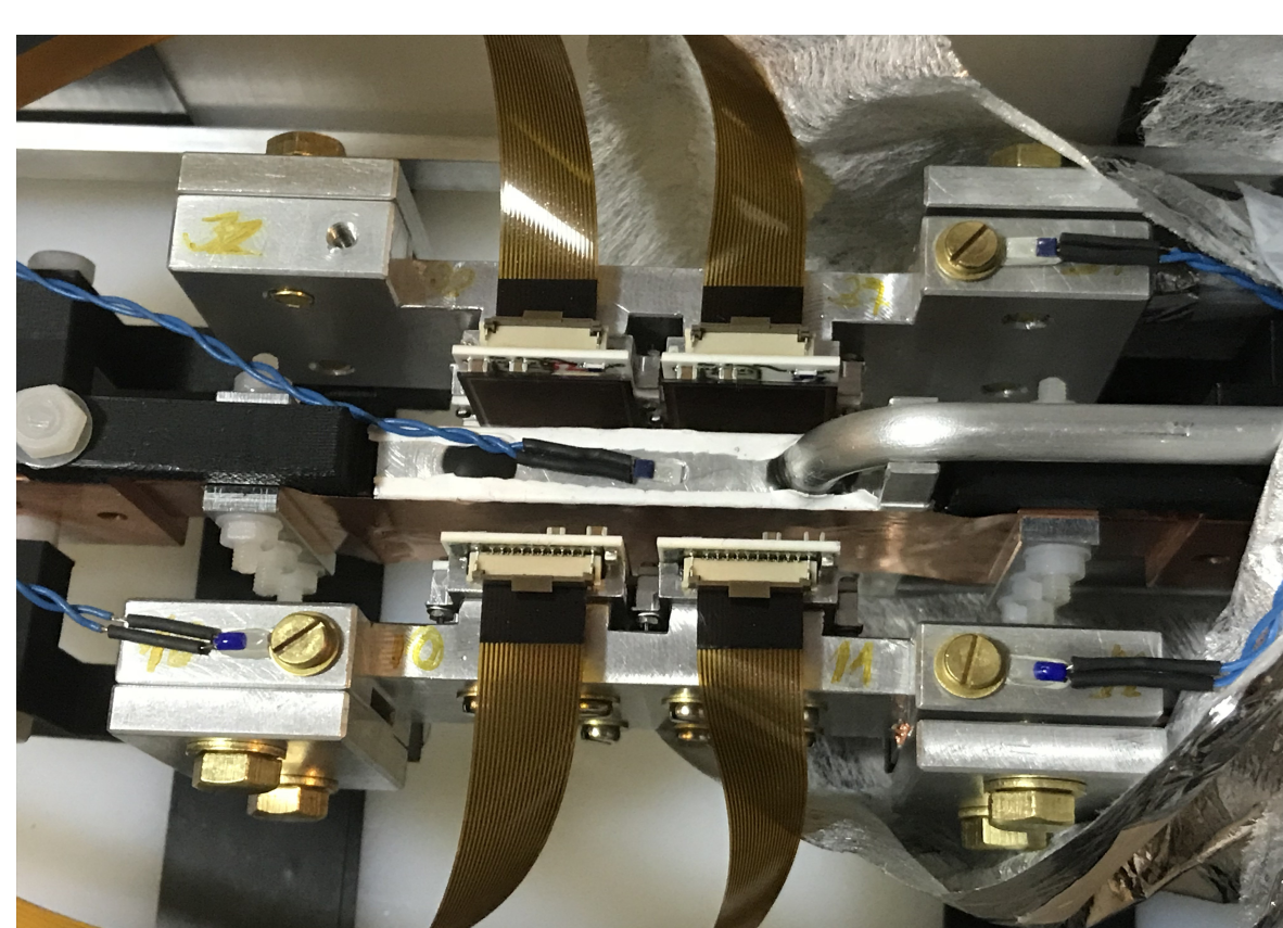
The new Silicon Drift Detectors mounted close to the Cu target in the setup, with readout cables and water cooling to counteract the heating due to the high current.
