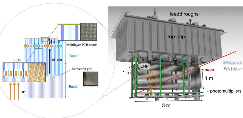
1. A charged particle crossing the detector produces electron-ion pairs and scintillation light.
