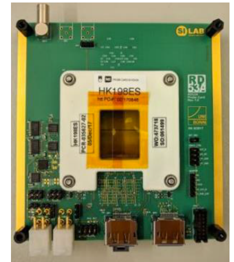
Needle card for wafer probing (developed in Bonn)
