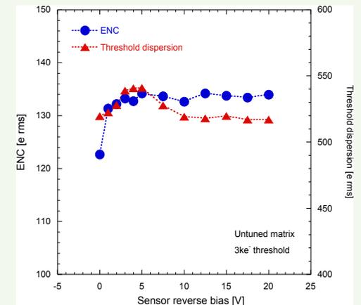
Main analog parameters have been investigated as a function of the sensor reverse bias voltage
