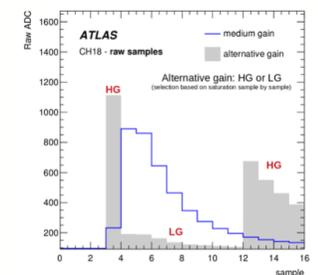
Sample-by-sample gain selection allows to output only the 2 gains which are relevant
