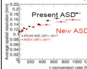
Average drift tube spatial resolution with **present** and **new ASD** as a fct. of the  $\gamma$  count rate. The higher gain of the new ASD reduces time-slewing esp. at high  $\gamma$  rates.
