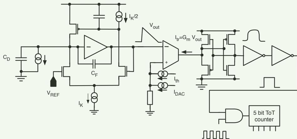
Schematic diagram of the asynchronous front-end integrated in the CHIPIX demonstrator
