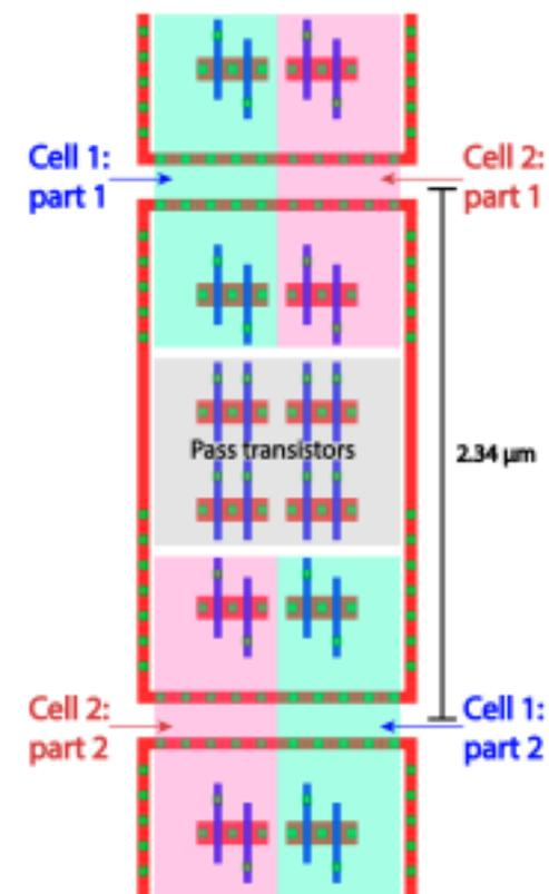
**RH-CAM layout in 28 nm CMOS technology (two interleaved cells)**
