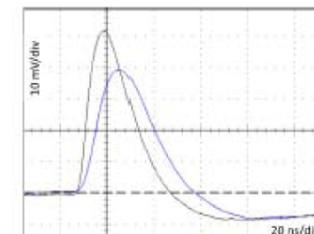
Signal peaking time of 12 ns **without** capacitive load as required (**with 60 pF** capacitive load 15 ns). Typical capacitance load of ATLAS MDTs 30 pF. The gain of the new chip is increased by a **factor 2**.
