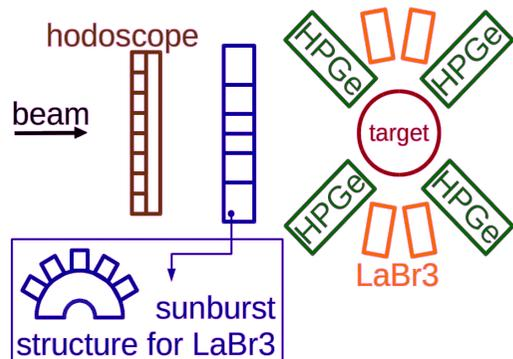
high energy resolution spectroscopy: study of X-ray emission of decaying muonic atoms in metallic artifacts - internal composition analysis with good depth resolution via beam momentum tuning
