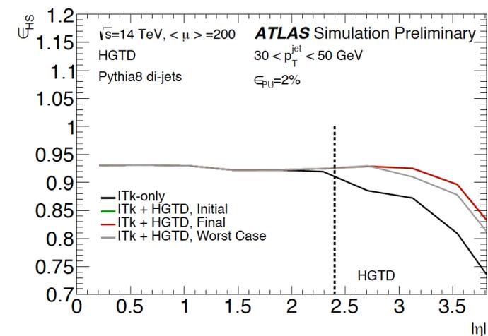
The proposed High Granularity Time Device (HGTD) improves the pile-up jets rejection in the forward region, degraded due to the vertex merging and larger track impact parameter resolution.
