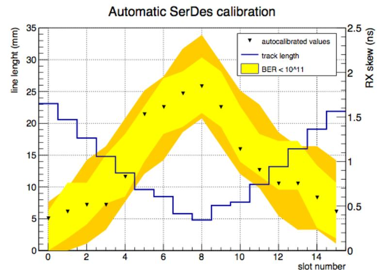
The calibrated delay values anticorrelate well with backplane track length. The Bit Error Rate contour is shown in yellow for comparison.
