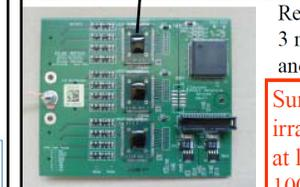
Readout board with 3 new ASD chips and a TDC chip.
