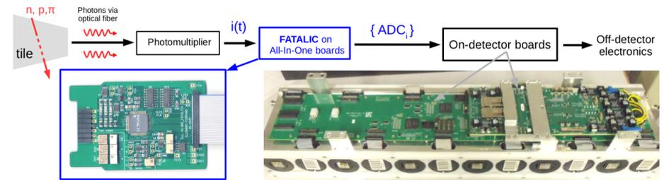
The light produced by tiles is converted by a photo-multiplier (PM) into electric current  $i(t)$ , which is processed by the *readout electronics* sending ADC counts to the rest of the chain.
