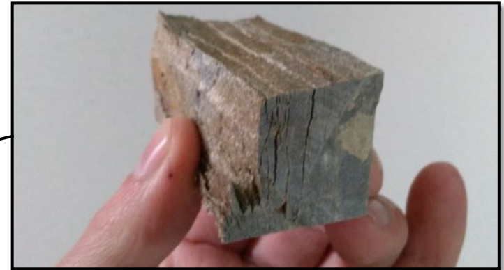
Micaschist - Paragneiss - Quartzite UCS: 9.9/8.8 MPa
