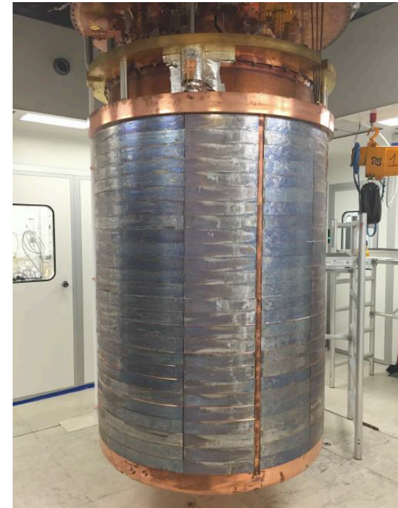
Lead shield installed
