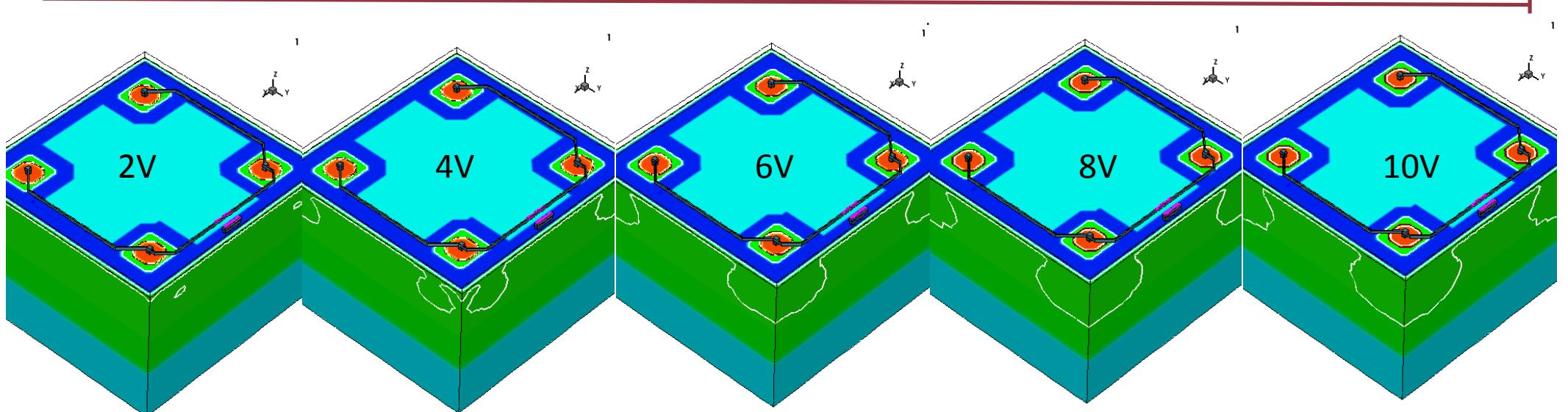
*Single pixel field: DC Vbias 2 to 10V, without back contact*
