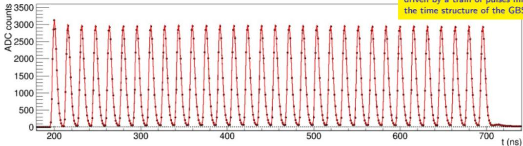
Detector response when the laser is driven by a train of pulses mimicking the time structure of the GBS
