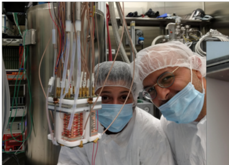
First setup equipped with SiPMs designed for DarkSide
