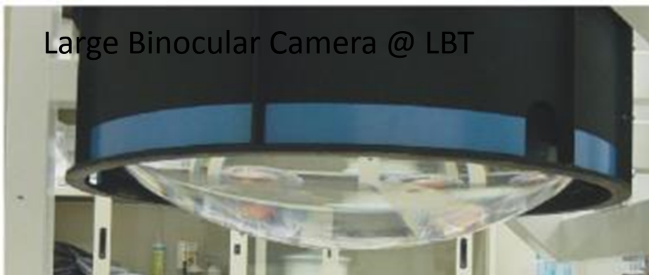
Large spheric meniscus lens D = 810 mm (120Kg)
