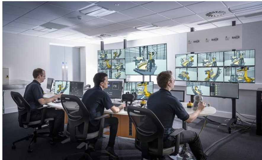
Figure - The RACE control room with VR screen, haptic devices with force feedback and supervisory systems
