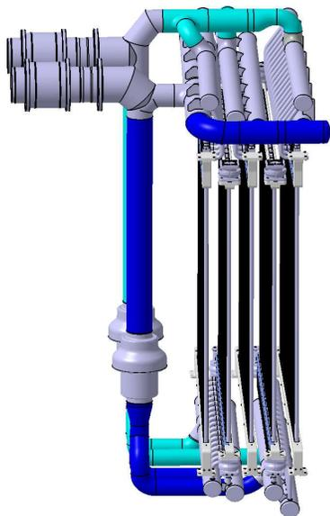
Five CuCrZr walls separate four channels where H-/D<sup>-</sup> and H<sup>+</sup>/D<sup>+</sup> ions are deflected by electrostatic fields.
