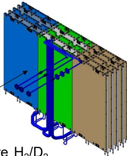
Five OF Cu walls forming four channels where H<sub>2</sub>/D<sub>2</sub> is injected for ion beam neutralization
