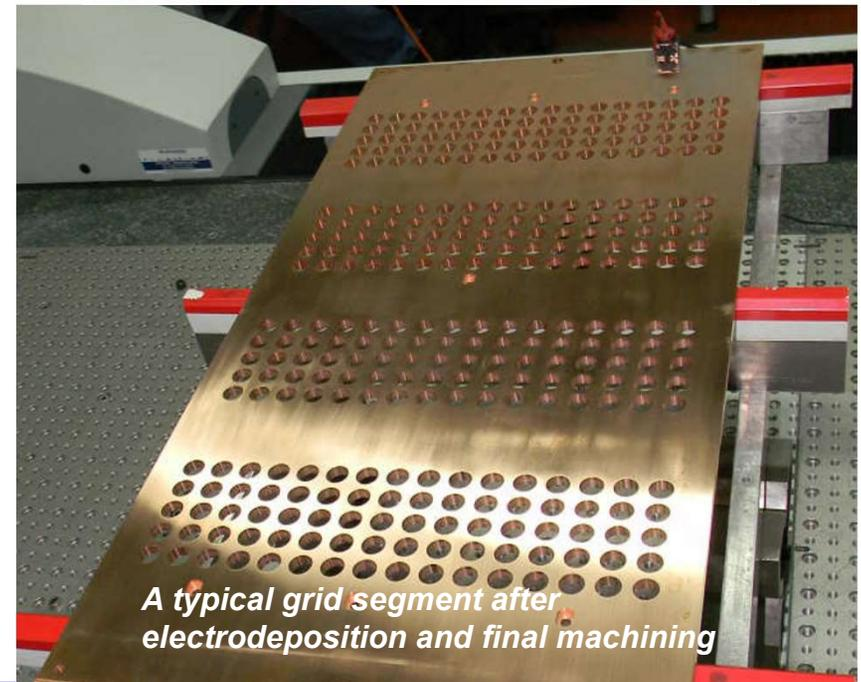
A typical grid segment after electrodeposition and final machining
