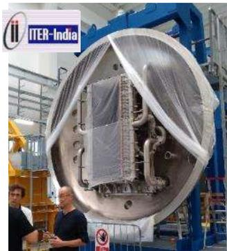
**Beam Dump for long pulses (up to 1 hour)**
