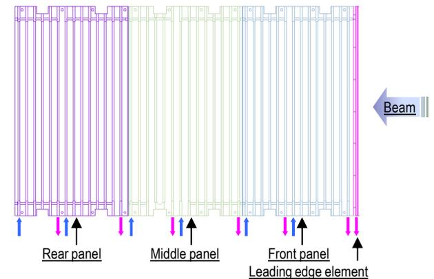
Ø18 cooling channels are deep drilled on 34 mm thick OF Cu plates.
