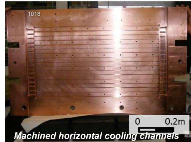
Machined horizontal cooling channels
