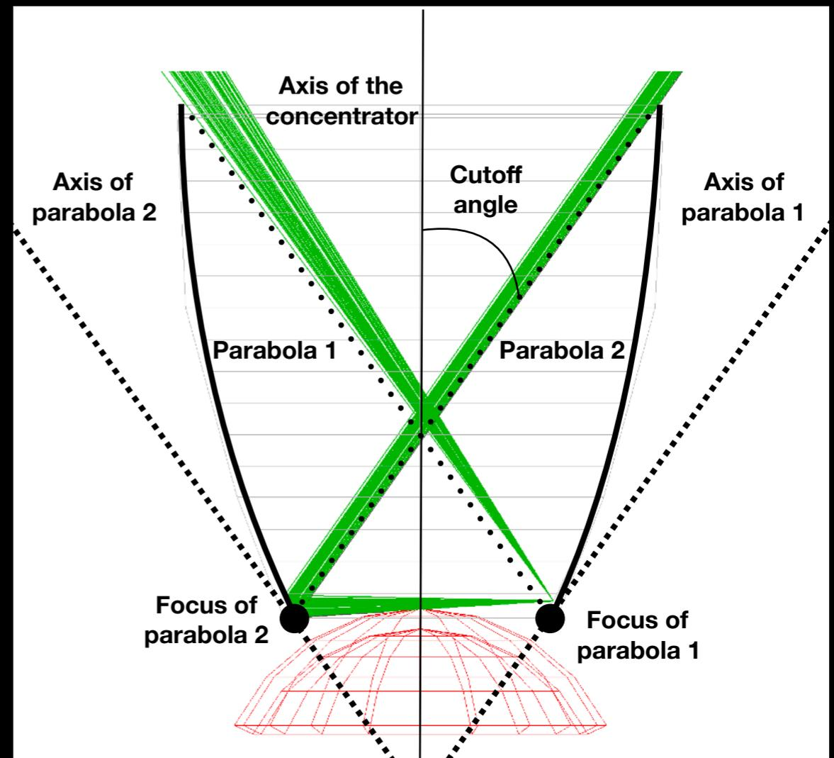
Geometry of a light concentrator and photon behavior in case  $\alpha > \alpha_c$
