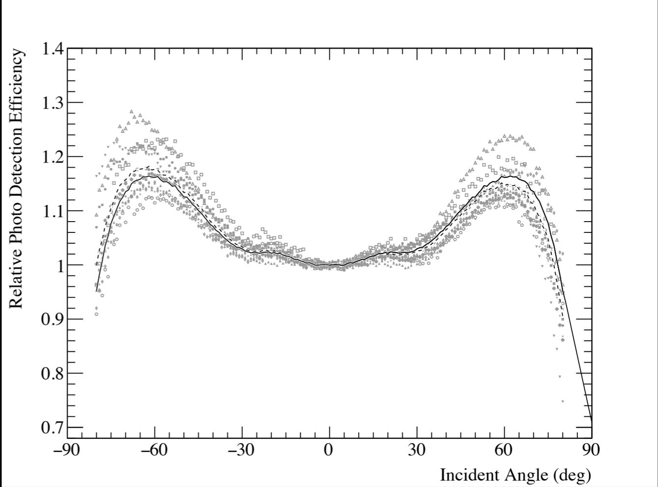
PMT relative detection efficiency
