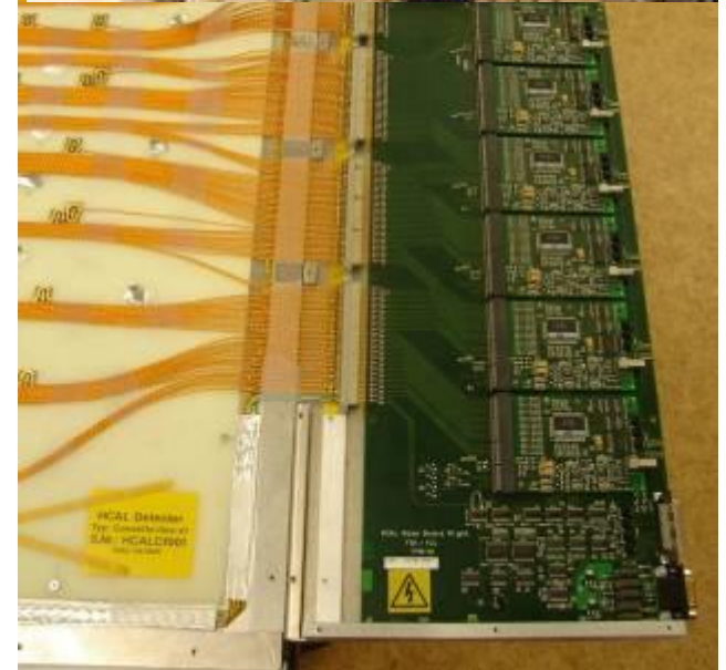
Mechanics and front end boards: DESY SiPM : Mephy Pulsar Moscow Front end ASICs: LAL
