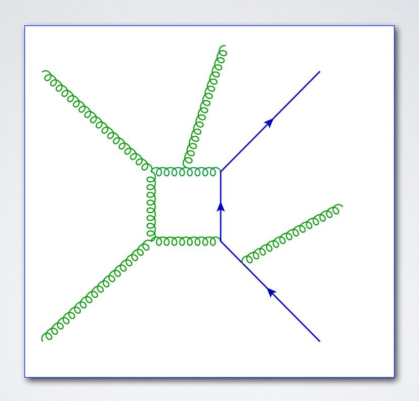
A diagram contributing a real-virtual NNLO correction to t-tbar-jet production
