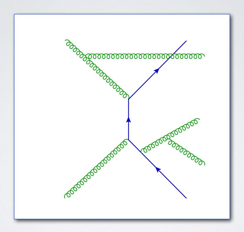
A diagram contributing a double-real NNLO correction to t-tbar-jet production
