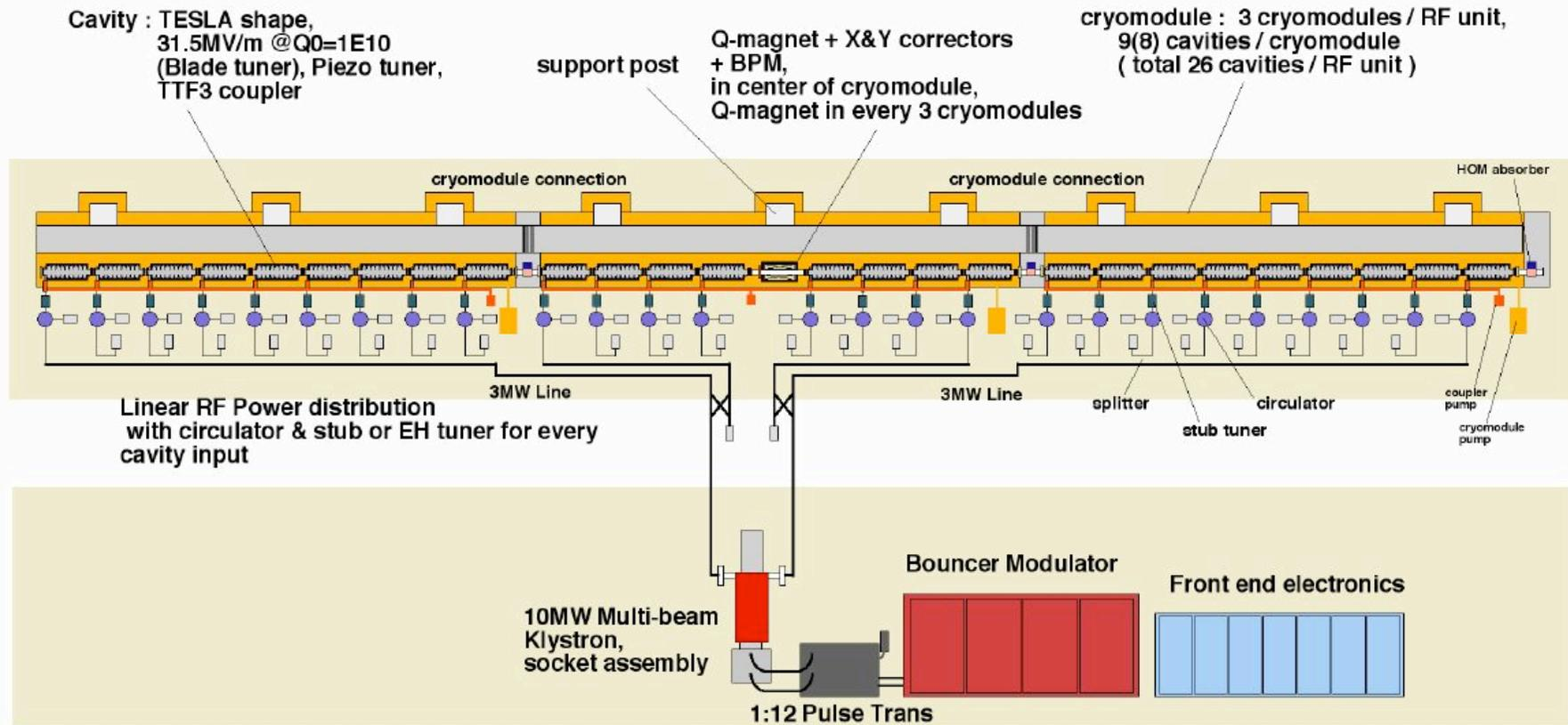
RF power system limits 33MV/m operation.
