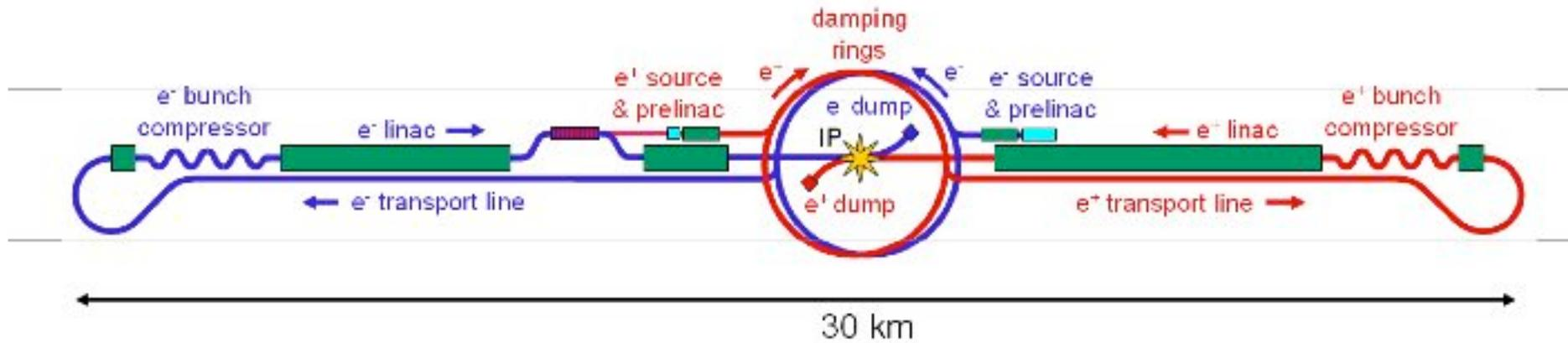
Two 6.5 km, 5 GeV damping rings in a shared tunnel around the interaction region
