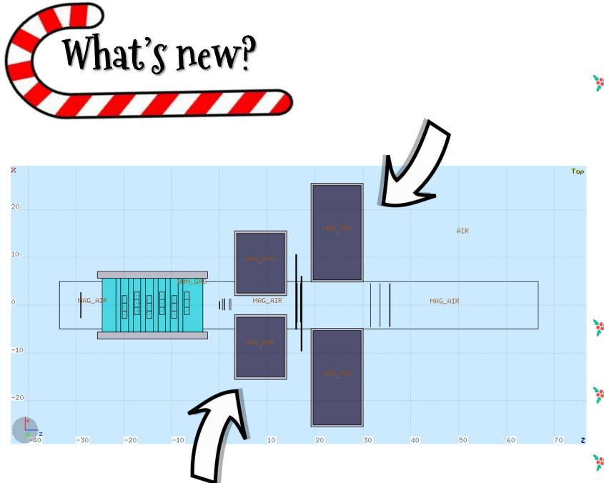
New magnets configuration: 🏋 11 cm long 🍹 5 cm distance Mag1: R<sub>in</sub>=2,5cm, R<sub>out</sub>=15,5cm, B<sub>max</sub>=13kG Mag2: R<sub>in</sub>=5,3cm, R<sub>out</sub>=25,5cm,  $B_{max}=8,7kG$ New distances btw the detectors of the magnetic system.
