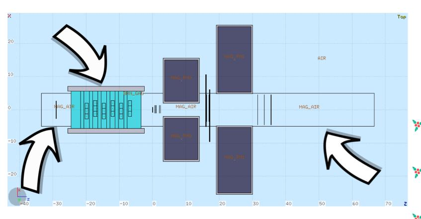
New magnets configuration: 🏋 11 cm long 🍹 5 cm distance Mag1: R<sub>in</sub>=2,5cm, R<sub>out</sub>=15,5cm, B<sub>max</sub>=13kG Mag2: R<sub>in</sub>=5,3cm, R<sub>out</sub>=25,5cm,  $B_{max}=8,7kG$ New distances btw the detectors of the magnetic system. Magnetic area extended to the
