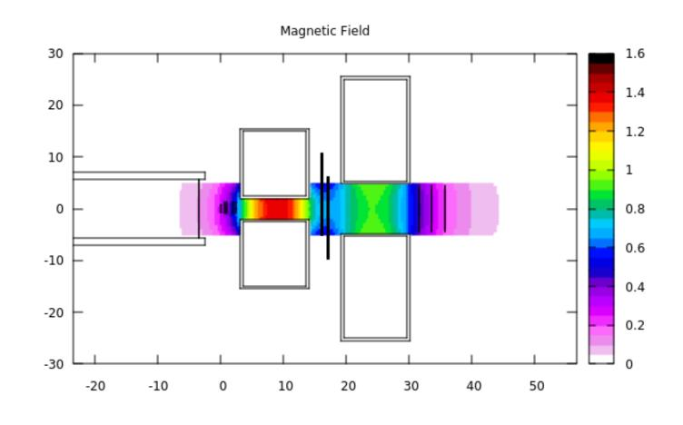
New magnets configuration: 🏋 11 cm long 🍹 5 cm distance Mag1: R<sub>in</sub>=2,5cm, R<sub>out</sub>=15,5cm, B<sub>max</sub>=13kG Mag2: R<sub>in</sub>=5,3cm, R<sub>out</sub>=25,5cm,  $B_{max}$ =8,7kG New distances btw the detectors of the magnetic system. Magnetic area extended to the beam monitor and the start counter.
