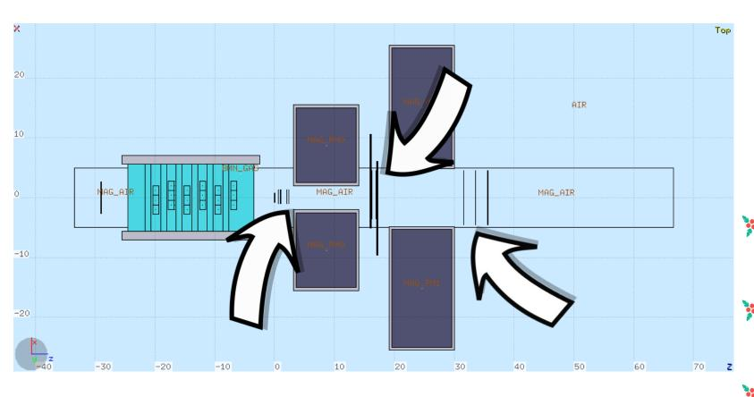
New magnets configuration: 🏋 11 cm long 🍹 5 cm distance Mag1: R<sub>in</sub>=2,5cm, R<sub>out</sub>=15,5cm, B<sub>max</sub>=13kG Mag2: R<sub>in</sub>=5,3cm, R<sub>out</sub>=25,5cm, B<sub>max</sub>=8,7kG New distances btw the detectors of the magnetic system. Magnetic area extended to the beam monitor and the start counter.
