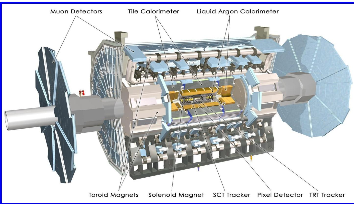
Detector is ready for data taking, waiting for LHC delivery of first collisions
