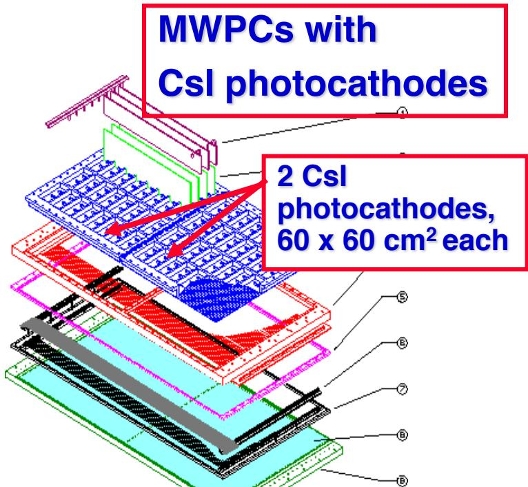
8 chambers, 5.5 m<sup>2</sup> in total; the largest CsI MWPC system in operation so far
