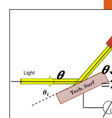
Decreasing of reflectivity at  $\theta_{i\downarrow i}=1^\circ$  is due to the achievement of the critical angle.
