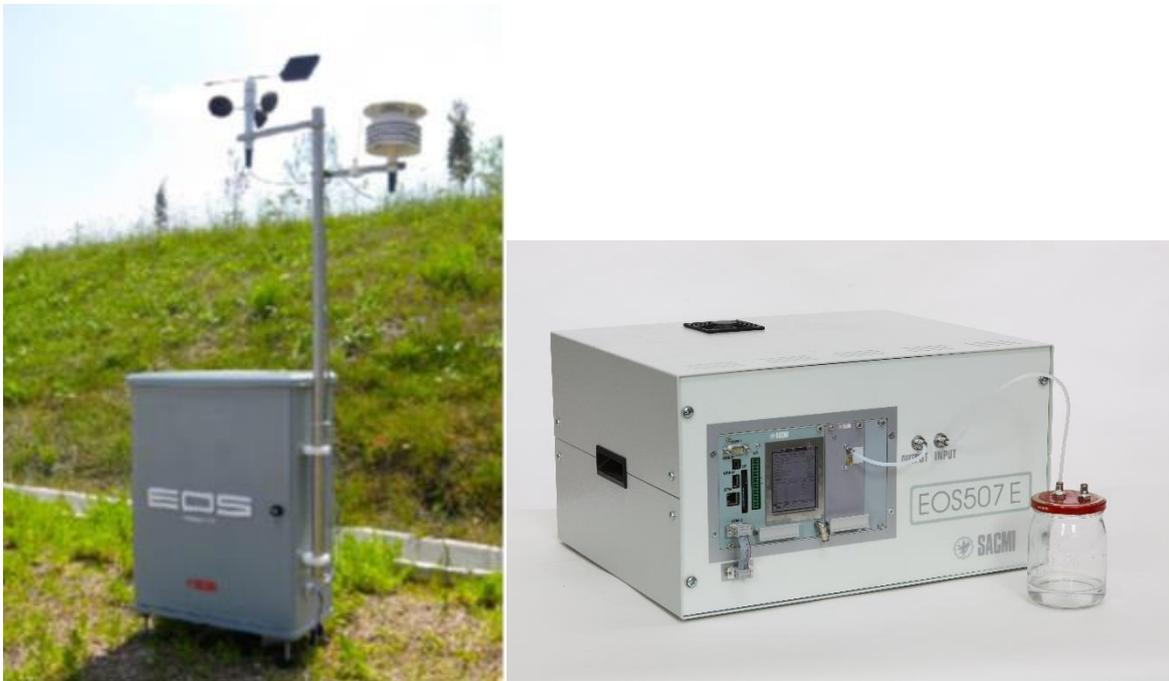
**Figure 2.** SACMI Electronic Olfactory Systems for outdoor (**left**) and laboratory (**right**) use.
