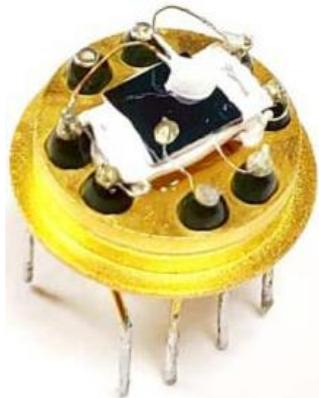
**Figure 1.** Capacitor sensor’s photo assembled with film resistive heater and thermistor. Package type is TO-8 (11 mm in diameter).
