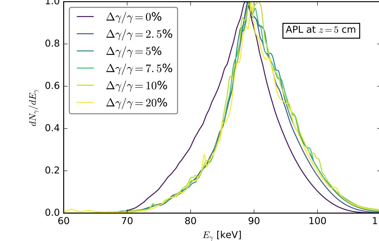
Figure 10: APLs allow for spectral filtering of Thomson spectra
