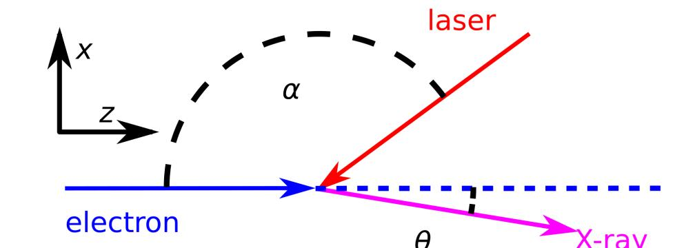
Figure 4: Geometry of Thomson scattering
