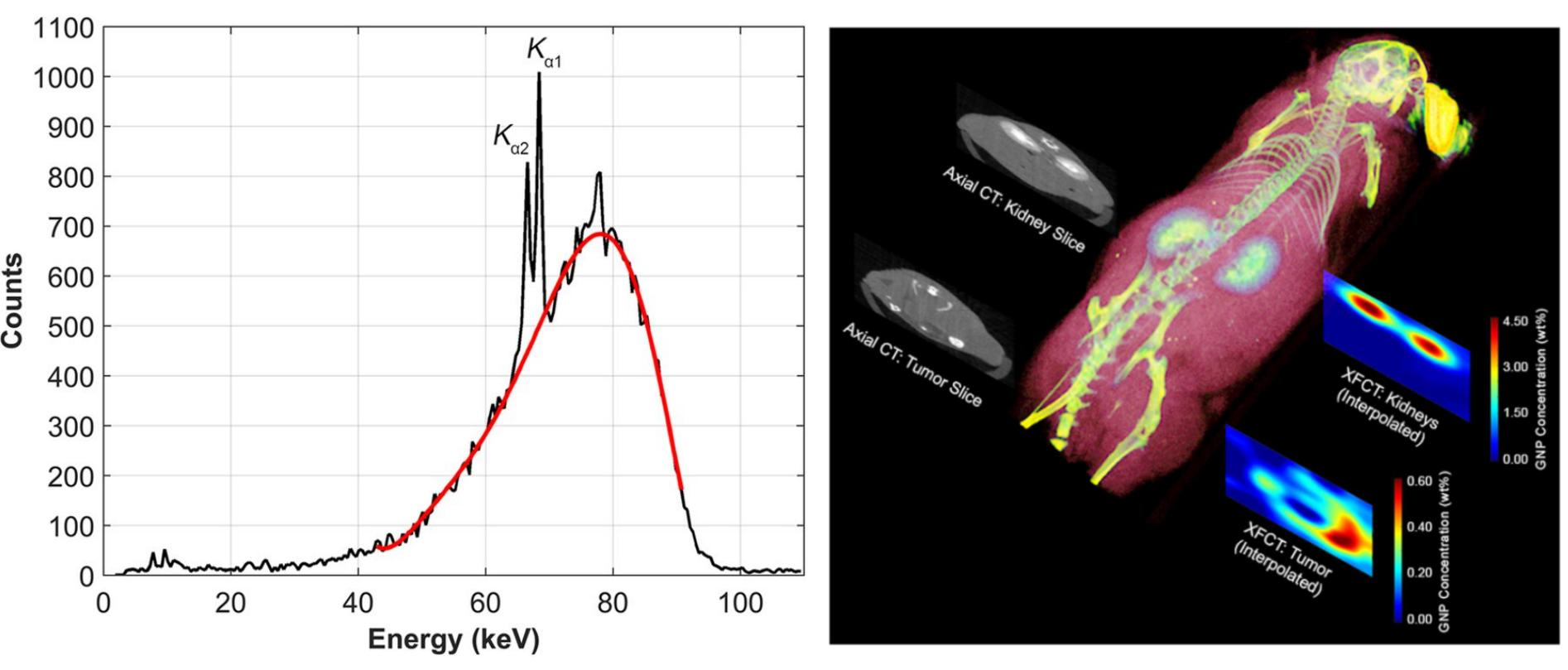
Figure 2: X-Ray tube spectrum with XFI signal [4]
