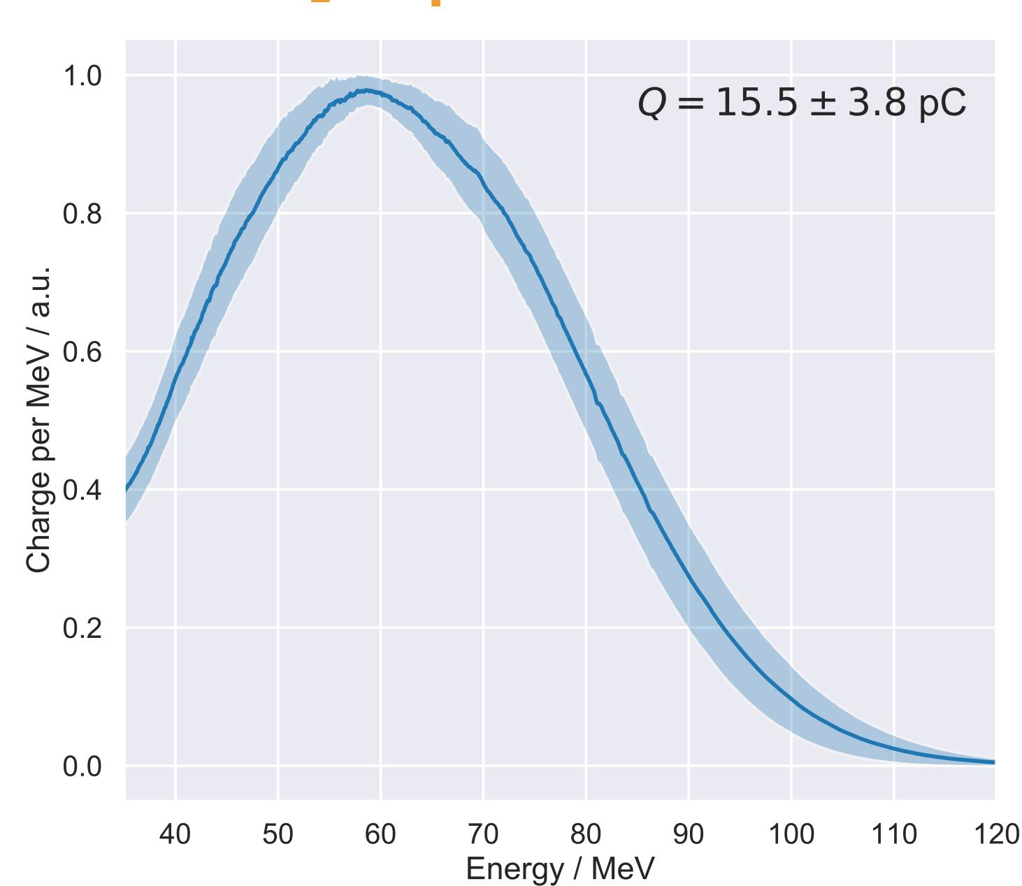
Figure 7: Average spectrum of the shots, showing high stability
