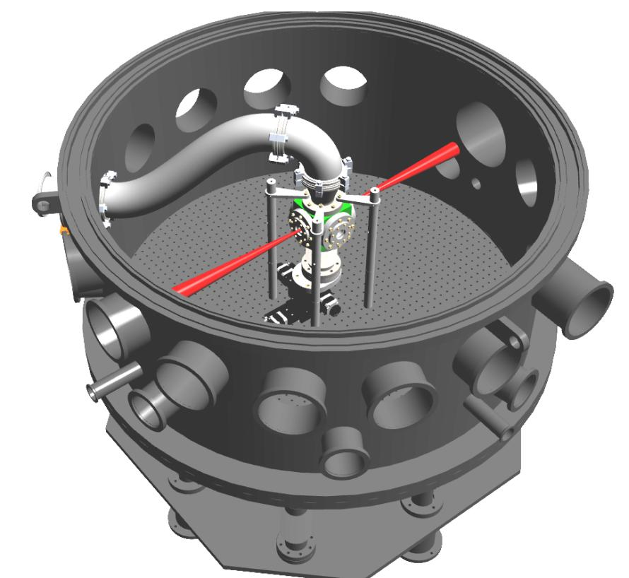
Figure 11: CAD rendering of the differential pumping cube
