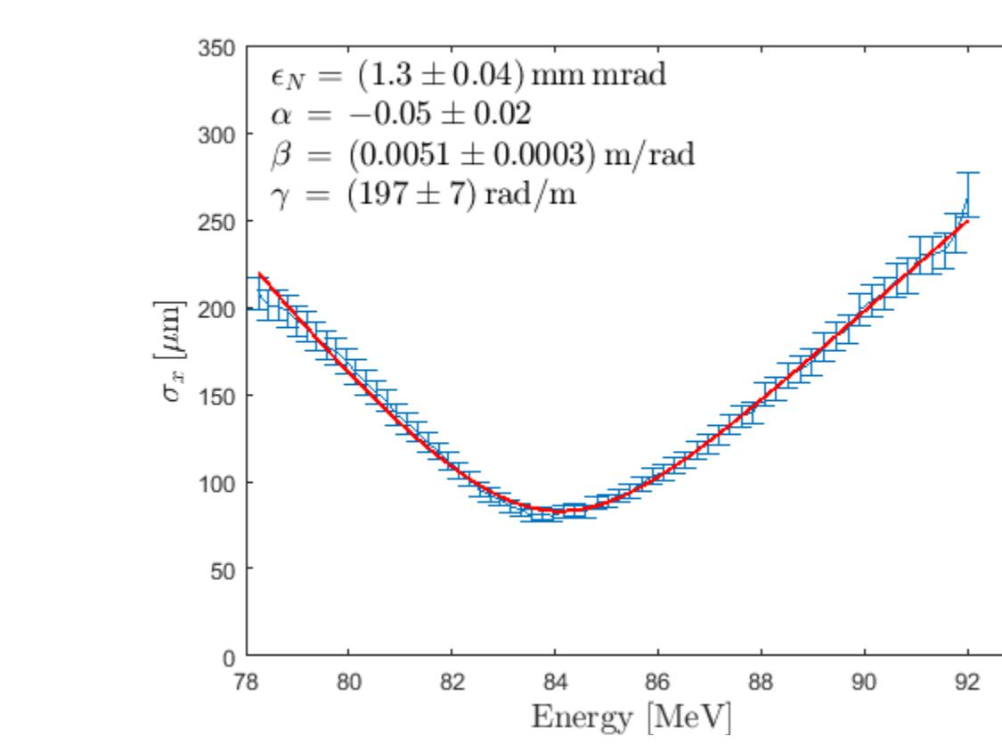
Figure 9: Emittance extraction from "butterfly" measurement
