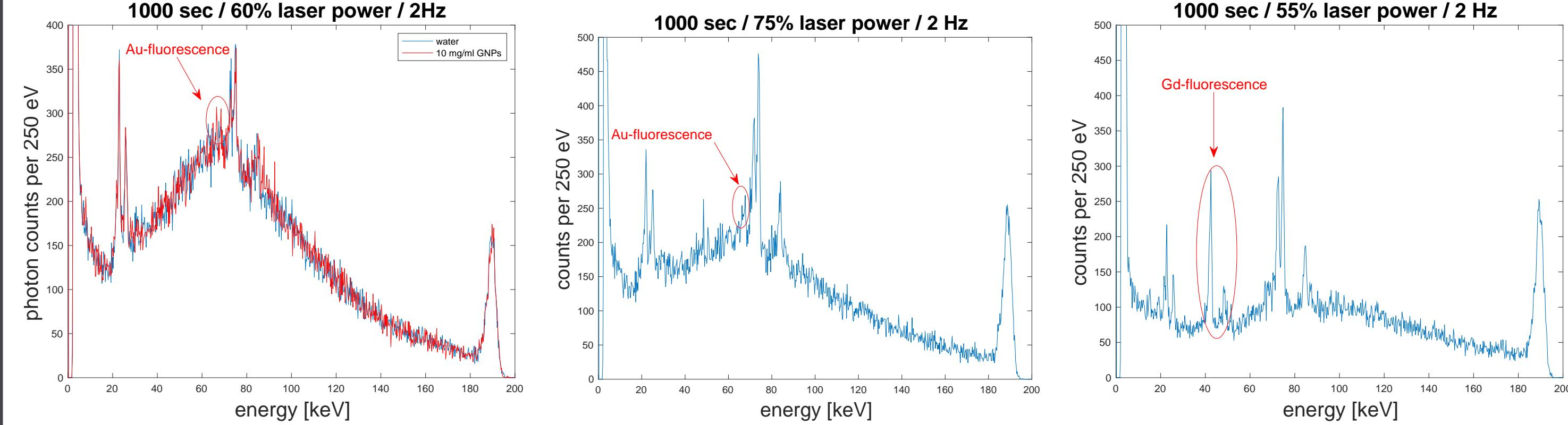
Figure 13: XFI signal and background, showing clear signal for Au measurement
