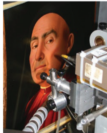
Example of PIXE to analyze the pigment's composition of The Trivulzio portrait by Antonello da Messina
