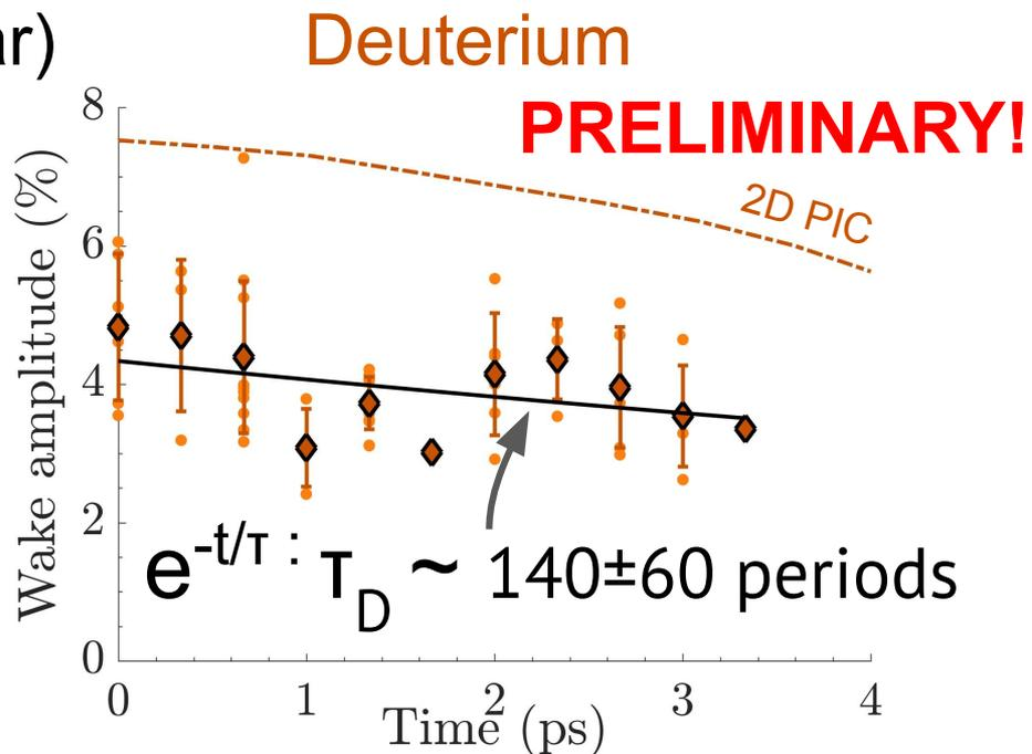
Simulation: 2D PIC (SMILEI), same design parameters as experiment (no free parameters!). *4 particles per cell*
