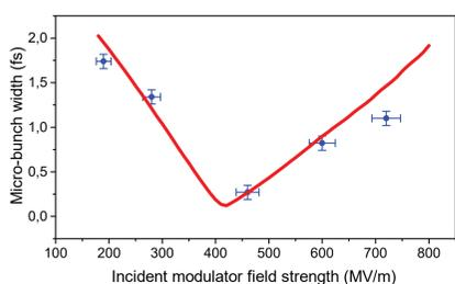
Simulation results (red curve) and experimental results (blue points) for the micro bunch length as a function of incident modulator field strength
