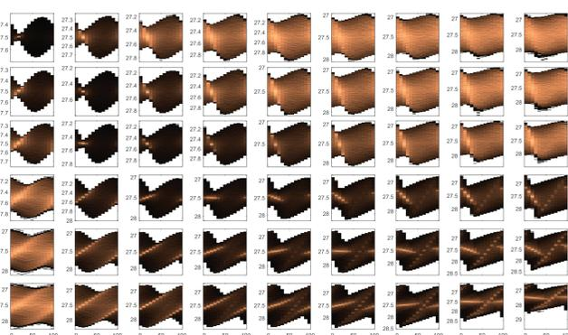
Simulations of diverse combinations of modulator and analyzer peak field. The relative phase between the driving modulator and analyzer field is scanned. The resulting spectrograms show characteristic and unique features. The experimental data is matched via the width and slope of the high density feature.
