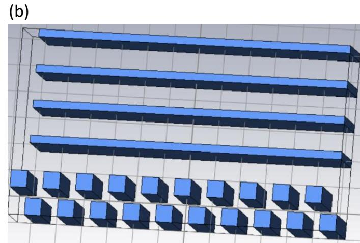
(a) Cylindrical and (b) cuboid shaped dielectric structures. It's a dual pillar with 4 Bragg reflectors.
