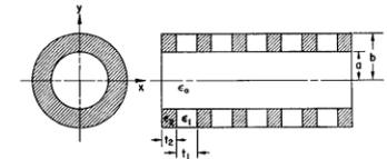
Fig. 1. Geometry of an anisotropic-dielectric-lined circular waveguide. The anisotropic dielectric is simulated by using spaced lamination of two different isotropic dielectric disks.
