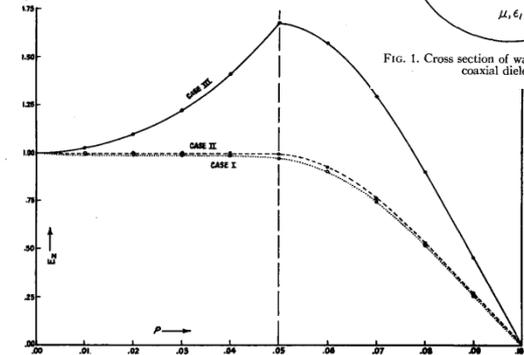
FIG. 1. Distribution of the longitudinal component of electric field strength through a cross section of the tube.
