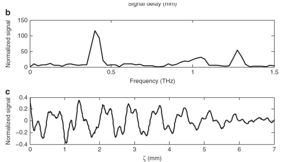
**Unusual sharp fall off in field strength—the pulse is too short. Expected 18 mm, measured – 5 mm at ~ 1 GV/m range. High field induced conductivity at THz ?**
