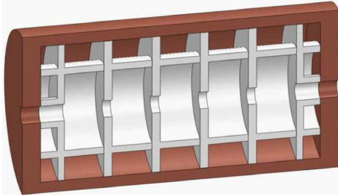
The DAA structure has high quality factor and a very high shunt impedance at room temperature since the electromagnetic field distribution of accelerating mode can be controlled by dielectric parts so that the wall loss on the metallic surface is greatly reduced: C-band (5.712 GHz),  $Q_0 \sim 119,314$  shunt impedance  $\sim 617 \text{ M}\Omega\text{m}$ ,  $TM_{02}$  mode.
