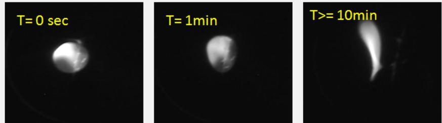
Beam test under 200 kV DC gun. The regular ceramic is charged < 1 sec. The DC beam test of the new ceramic demonstrated its self-discharge during ~ 1 hour test.
