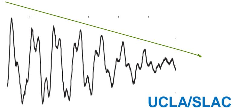
the observed damping in experiment is much larger than that ascribable to dielectric or metallic losses under the conditions used in these experiments. This damping is an unexpected feature—comparison with previous studies makes it clear that the observed damping is introduced by use of a very intense, short pulse electron beam.
