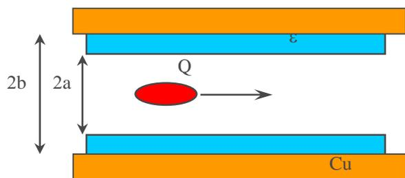
Low-loss high breakdown strength ceramic for the dielectric structures
