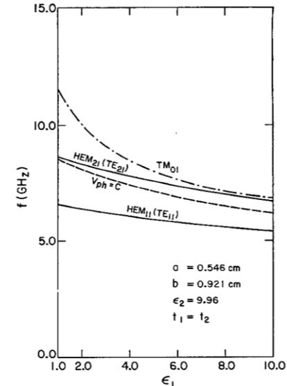
Fig. 3. The changes of cutoff frequencies of HEM<sub>11</sub>, HEM<sub>21</sub>, and TM<sub>01</sub> modes and the operating frequency of HEM<sub>11</sub> mode at  $v_{ph} = c$  (the dashed curve) with  $\epsilon_1$ .
