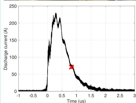
The discharge circuit prototype we have realized provides currents up to 600 A with a capacitor bank of  $C = 10.8$  nF in series with a resistance  $R = 7 \Omega$ . The core is represented by a HV thyristor switch providing up to 12 kA peak current when operating at 44 kV voltage. A second capacitor is used as a low-pass filter and cut the high-frequency ( $f > 40$  MHz) oscillations. Two HV diodes prevent negative current overshoot and protect the HV switch.
