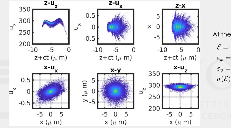
At the end of the plateau  $\mathcal{E} = 150 \text{MeV}$   $\varepsilon_x = 0.21 \text{mm} \times \text{mrad}$   $\varepsilon_y = 0.23 \text{mm} \times \text{mrad}$  $\sigma(\mathcal{E})/\mathcal{E} = 1.6\%$
