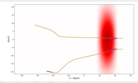
Tracked particle longitudinal momentum in the fully PIC and Envelope scheme
