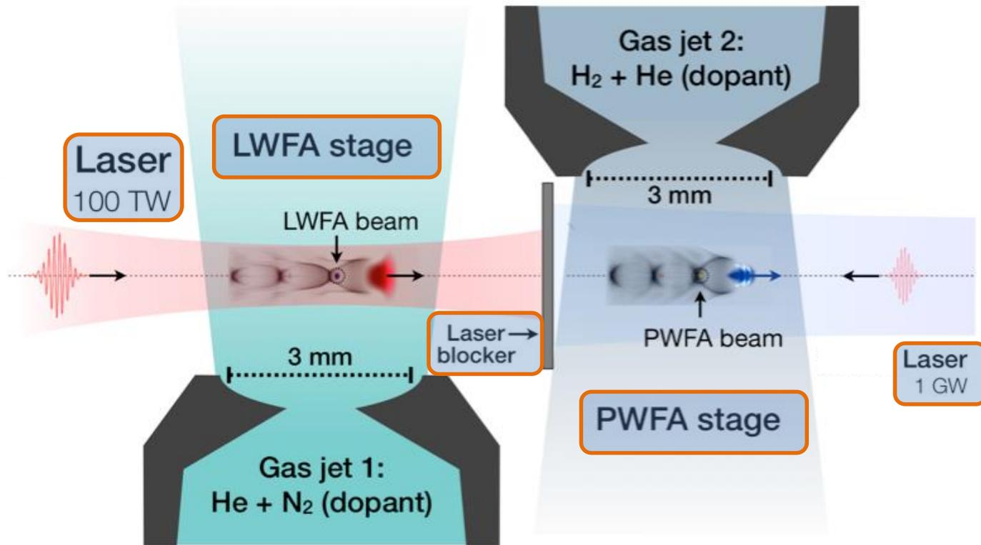
~0.5 nC injection via self-truncated ionization injection
