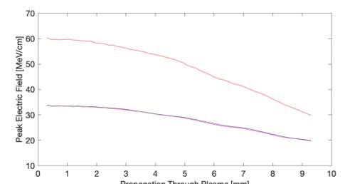
**Fig. right:** Peak of the longitudinal electric field in MeV/cm. The higher dense simulation has an electric field twice as high as the other two simulations as expected, however it decreases faster.
