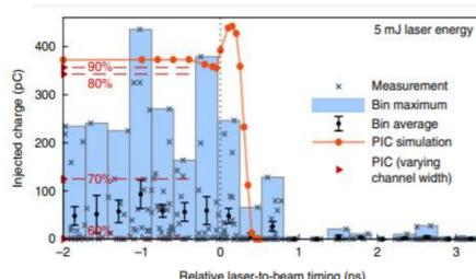
Laser timing scan at 5mJ injector laser energy
