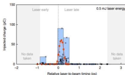
Laser timing scan at 0.5mJ injector laser energy
