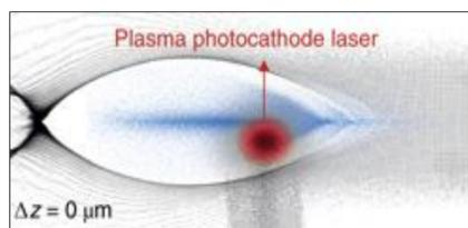
3D PIC simulation of 90 plasma photocathode injection
