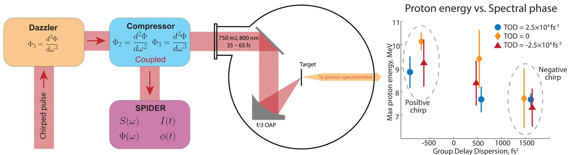
Positive chirp of the pulse gives higher proton energy compared to negatively chirped or transform limited pulse. TOD = 0 (symmetric pulse) results in highest proton energy for each pulse duration.
