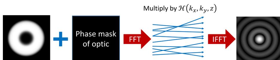
Flow chart illustrating how the ASM numerical code works for each wavelength.
