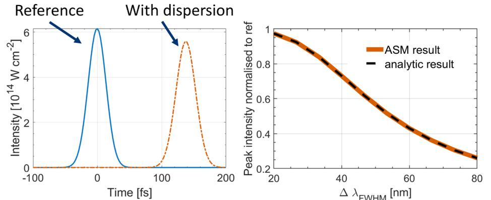
Temporal intensity profiles at focus for initial Gaussian beam with  $I_0 = 10^{11} \text{ W cm}^{-2}$ ,  $\lambda = 805 \text{ nm}$ ,  $\Delta\lambda_{\text{FWHM}} = 30 \text{ nm}$  (left). Axicon parameters;  $\alpha = 5.52^\circ$ ,  $t = 3 \text{ mm}$ , fused silica. Initial beam radius  $25.4 \times 0.1 \text{ mm}$ . Reference has  $n(\lambda) = \text{const}$ .
