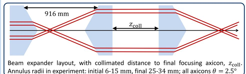
In experiment, focal spot quality was very sensitive to misalignments of the axicons in the expander. The effect of a small offset of the first axicon,  $\delta x_1$  is modelled below (all distances scaled down by 10).
