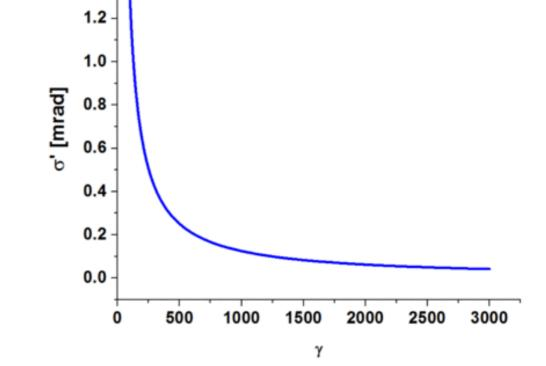
The divergence resolution as function of energy (i.e. relativistic  $\gamma$ ) is shown in this plot. Since at SPARC\_LAB the maximum beam energy is below 200 *MeV*, there is the need to have high divergence beam in the measurement point. Some data has been already acquired, as shown in next figure, but the divergence was  $\sigma_{x} \sim 0.1 \, mrad$ , below the resolution for beam with E = 160 MeV.
