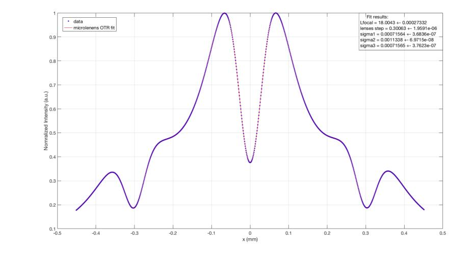
From the fit results the divergence of each lens is estrapolated; thus the quantities  $\langle x'^2 \rangle$  and  $\langle xx' \rangle$  in the emittance formula can be computed. By means of the spot, obtained by the beam transport (by the camera, for what concern the experimental setup), the normalized emittance, retrieved by the algorithm, is:
