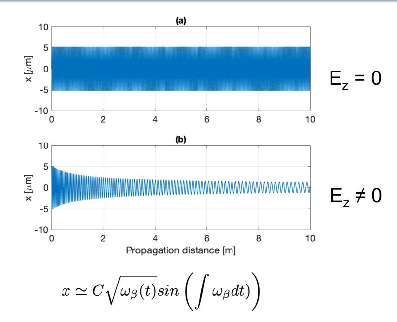
oscillations due to focusing forces from the ion column, governed by the equation:
