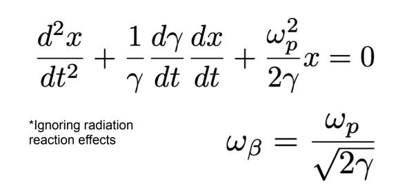
This motion has a linear sinusoidal solution in the case of constant energy and a decaying amplitude and betatron frequency for a non-zero accelerating field [2], via the WKB approximation
