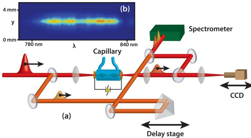
Measure the spectrum of two broad-band pulses with time delay  $\tau$ :
