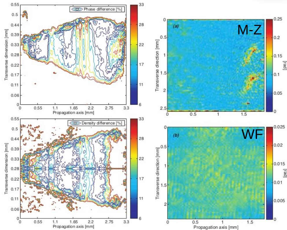
The difference in the measured values is 10-20%. The base noise averaging over 188 maps is 95.7 mrad for the modified M-Z and 11.4 mrad for the WF sensor
