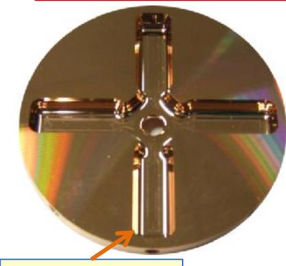
HOM damping waveguide
