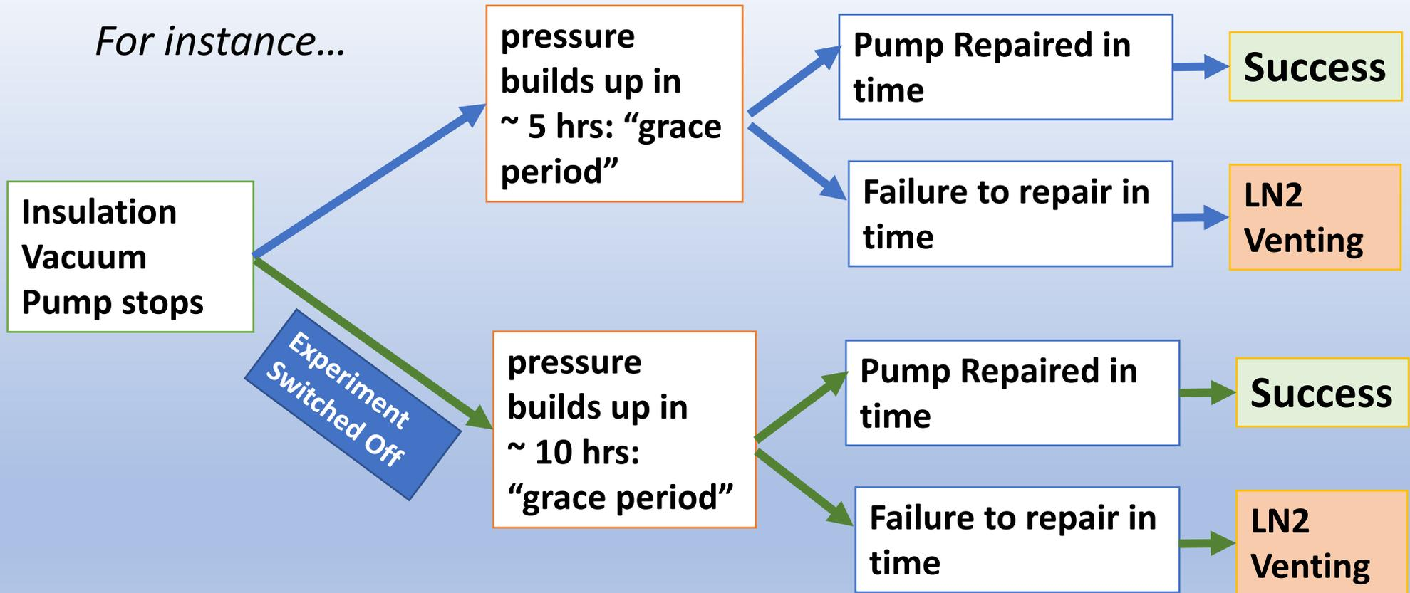
*Of course, the grace period can vary from days (e.g. pumps stop with solid N<sub>2</sub> inside) to minutes, if a gasket fails.*
